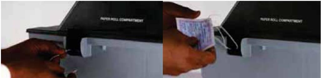
After installation of paper roll in the paper roll compartment of VVPAT, seal the latches of Paper Roll Compartment by passing a thread through holes provided on the latches using Address Tag showing the particulars of the election with the seal of the RO.
