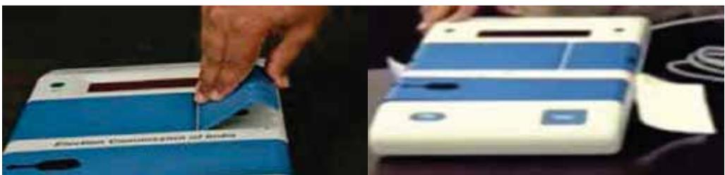
After Candidate set, seal cover of the Candidate Set Section of CU by passing a thread through hole provided on the right side using address tags showing the particulars of the election with the seal of the RO.
